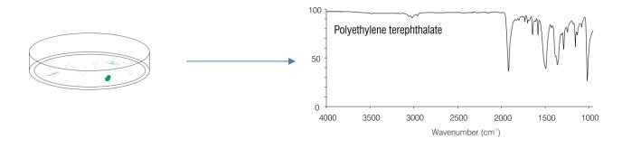
Chemical characterisation of MPs is most commonly achieved through IR spectroscopy: FT-IR and Raman.
